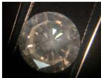
Fig. 3.5.5.6 Diamond with shallow pavilion depth causes light leakage thus no brilliance
