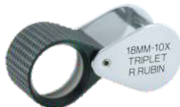
Fig. 4.1.11.3 Triplet 10X loupe 18mm Diameter from popular brands
